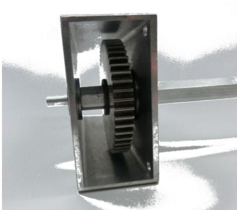
Step 6: Press an FR6 bearing into the middle hole of the motor side.
