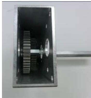
Step 9: Insert the small cluster gear with the flat side facing towards the large cluster gear.
