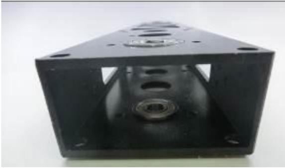
Step 12: Place the .51 x 1/2 PVC Spacer above the FR6ZZ bearing.
